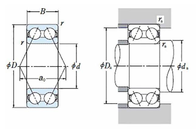
Double row steel shielded angular contact bearing from the world leader NSK, the worlds largest ball bearing manufacturer offering unparalelled quality
